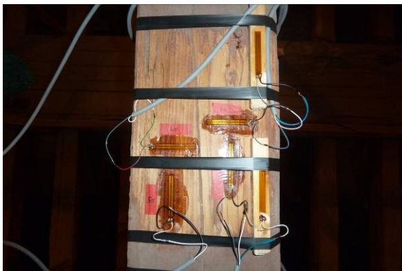
Fig. 4 The strain gauges installation and thermal isolation
