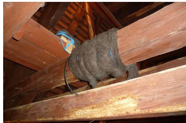
Fig. 4 The strain gauges installation and thermal isolation
